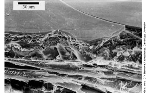
UNDER THE MICROSCOPE. Magnification of the surface layer of varnish (0.03mm) of a cello made by Pieter Rombouts, a contemporary of Antonio Stradivari.
