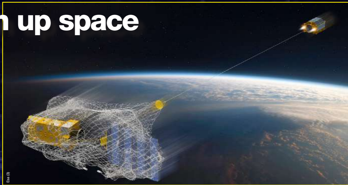
3 RemoveDebris: removing space debris by catching it with a net or harpoon. Successful in-orbit tests conducted in 2018 and 2019. University of Surrey project with a consortium of companies.
