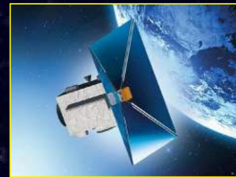
5 Adeo (Drag Augmentation Deorbiting Subsystem): sails system from 3 to 100 m 2 that pushes the disused satellite into a lower orbit to make it disintegrate. it is applicable to new satellites up to 1.5 tons of mass. Esa project.
