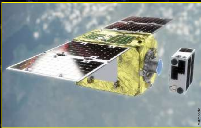
2 Elsa (End-of-Life Services Astroscale): mission of the Japanese space company Astroscale. It features a satellite equipped with a magnet to hook debris. A prototype was launched in March 2021.
