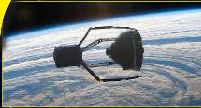
1 ClearSpace-1: a 100 kg probe with 4 robotic pincer arms to capture the Vespa, a part of the 112 kg Vega launcher. Esa project of 100 million euros with launch scheduled for 2025.
