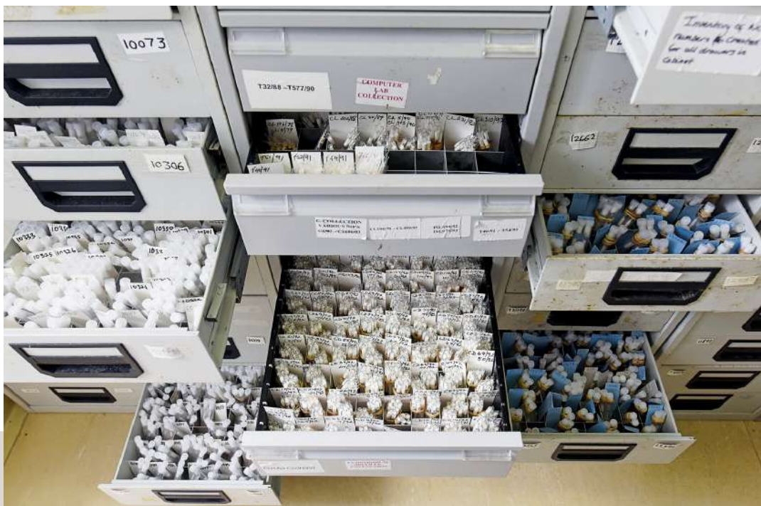
PREPARATION. Vials of bacteria in a dryer: without water they can be stored for many years.
